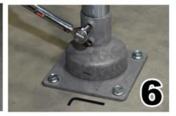
Insert both set screws and tighten to 100 ft. lbs. with a torque wrench or the provided 3/16" allen key to hold post securely in place
